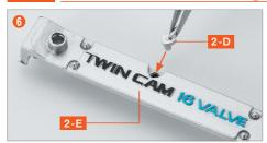
Insert the projection of the **Hose Connector 2-D** into the central hole of the
