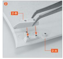
Turn **Hood 2-A** upside down and align the **Hood Hinge (L)2-B** with the screw holes in the positions as shown.
