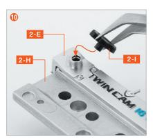
Turn the screwed assembly ① face up, and press the Oil Cap 2-I into the hole on 2-E at the position shown in the photo to fix it in place.
