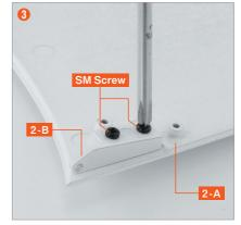
Once **2-B** is aligned, secure it at the two positions with **SM screws**. Use the screwdriver included in Issue 1.
