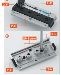
Once **2-F** is aligned as shown in photo the turn the entire assembly over, and fasten it at the two positions indicated in photo the using **SP screws**.
